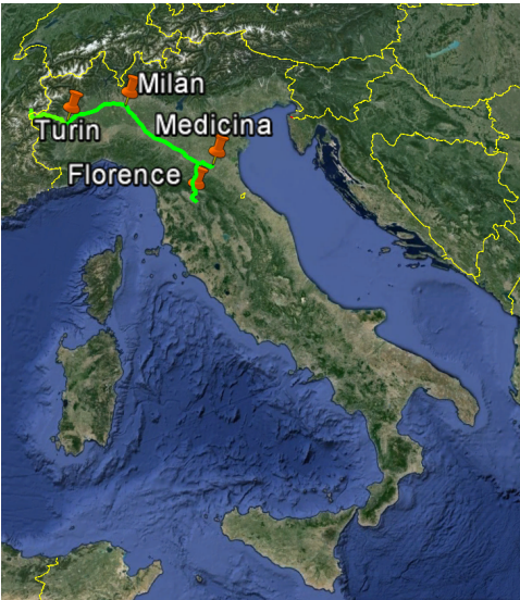
Fig. 1. The map of the present LIFT backbone. A single fiber link connects INRIM (Turin) to Bologna, in central Italy. Here the radiation is split: one of the arms connects INRIM to the European Laboratory for Non Linear Spectroscopy in Florence (total length 642 km); the other arm connects INRIM to Medicina Radiotelescope (total length 544 km).
