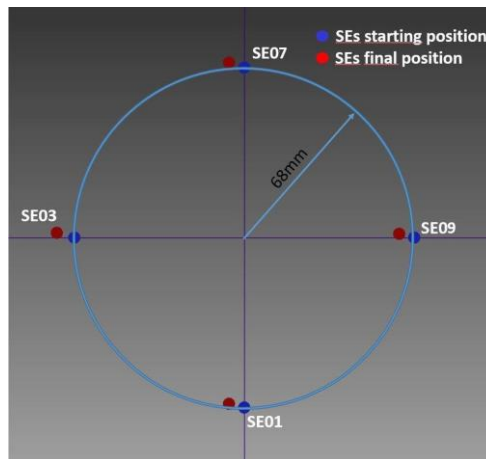
Figure 11: position of the SEs used for tip-tilt and focusing alignment of the AM, as seen from in front of the GWS entrance. The SEs were initially positioned on a cross pattern (blue circles) on a circle 68 \text{ mm} in radius, centered on the nominal center of the GWS focal plane. The pupils we got in these positions were highly defocused, so we moved the AM in focus, tracking the beam at the same time with the SEs. The red circles represent the positions of the SEs where we had, at a visual inspection, pupils with no defocus signal. The final positions of the SEs are shifted, on average, of 6 \text{ mm} in X axis and 2 \text{ mm} in Y axis wrt the starting position
