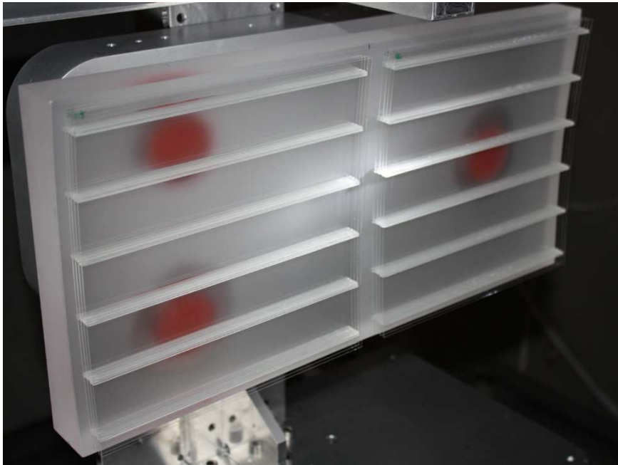
Fig. 1. An optical module, manufactured at INAF/OAB, made of four stacked pairs of slumped glasses (after Civitani et al. , 2013). Each pair is a grazing incidence parabola-hyperbola system operating two reflections in sequence. Ribs are used to properly space the mirrors and to endow them with the needed stiffness.
