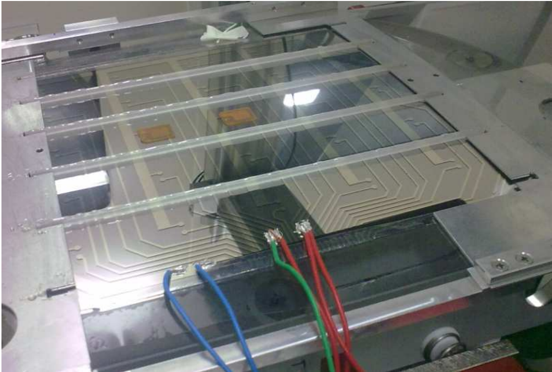
Fig. 6. The active glass foil prototype during the integration in the Integration Machine at INAF/OAB. The ribs are being glued while the optical surface is maintained in contact, via vacuum suction, with a precisely figured mould in BK7. The integration process is performed at a (20 \pm 0.1)^\circ\text{C} controlled temperature.
