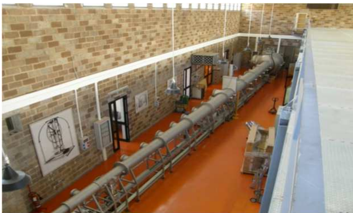
Fig. 9. The XACT X-ray facility in INAF/OAPA. A 35 m-long vacuum tube is used to illuminate with X-rays the samples in the vacuum chamber, visible in the background.
