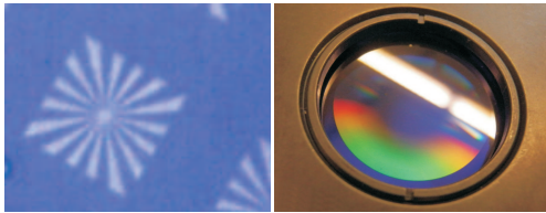
Fig. 2. Resolution test (left) and an f/1.5 Fresnel Zone Plate (right).
