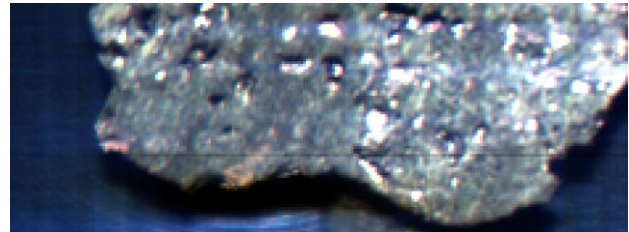
Fig.1. RGB image acquired with SPIM on the meteorite fragment (R:0.70 \mu\text{m} , G:0.53 \mu\text{m} , B:0.44 \mu\text{m} ).
