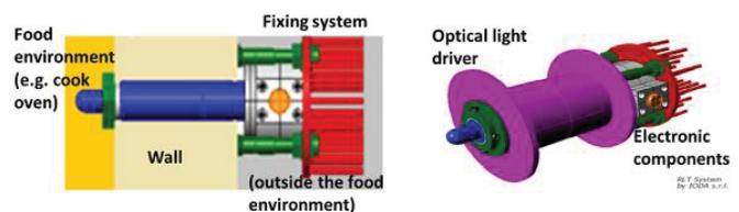
Fig. 1 Main components of the RLTProFood system and 3D representation.
