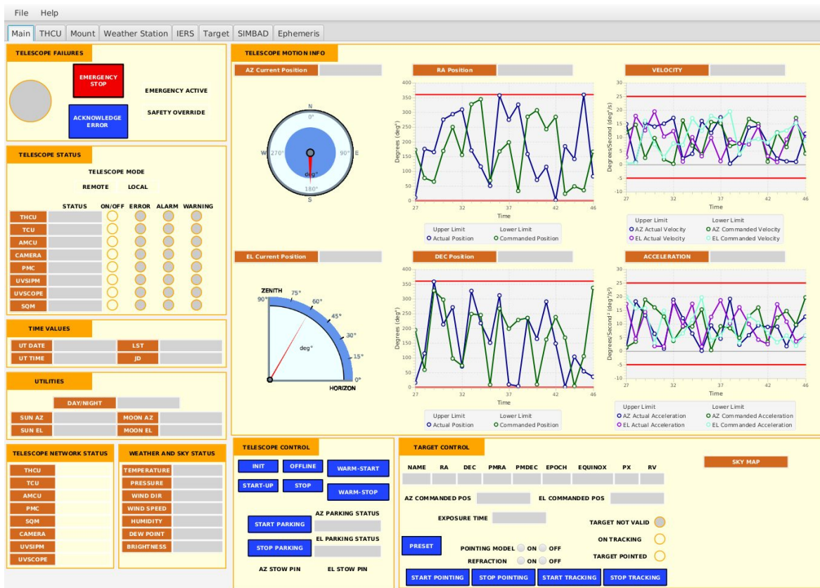
Figure 5. ASTRI Engineering GUI main view. This view allows the operator the control and monitoring of the most important functions of the telescope.
