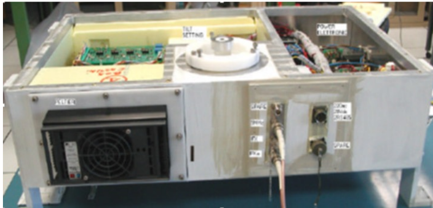
Figure 11: Internal view of the coaxial-feed receiver XKa- band during laboratory tests.
