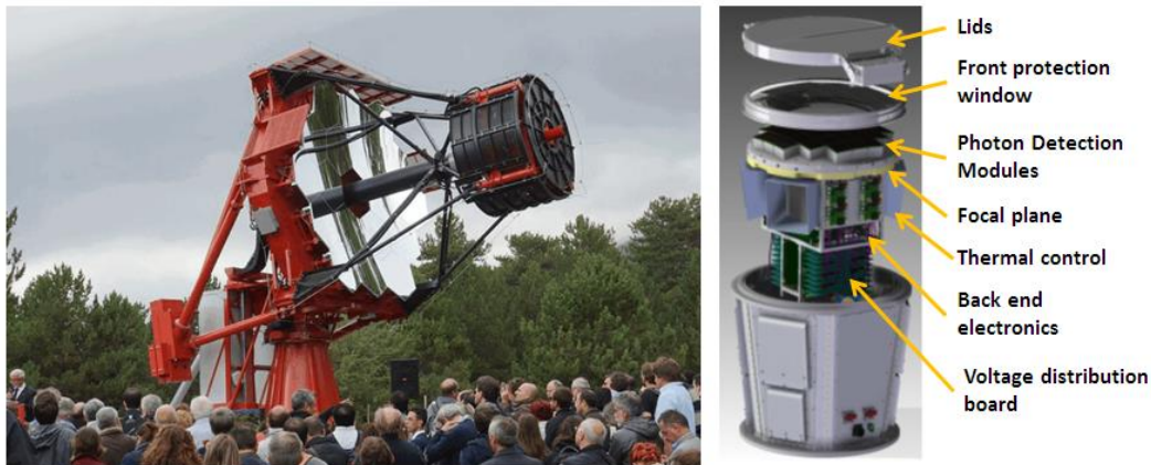
Fig.1 –The ASTRI SST-2M telescope prototype installed at the Serra La Nave (left) and exploded sketch of its camera (right).
