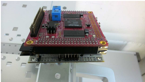
Fig. 7. Colibri board from Acme Systems connected to a SBC FOX Board G20.
