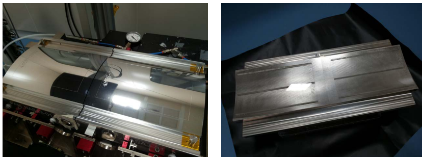
Figure 3: (A) the integration mold tandem for the 8.4 m focal length. The corresponding radius of curvature @IP is 485 mm. (B) The first integration trial based on the glass slumped by NASA.
