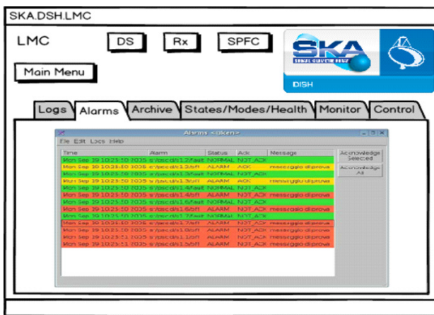
Figure 2: Sketch of a screen of DISH LMC engineering interface showing the alarm management UI.
