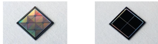
Fig. 6. The 2 \times 2 SDD array, composed of four 5 \times 5 mm 2 single cells. The left panel shows the anode side, while the entrance window for the scintillation light is shown in the right panel.
