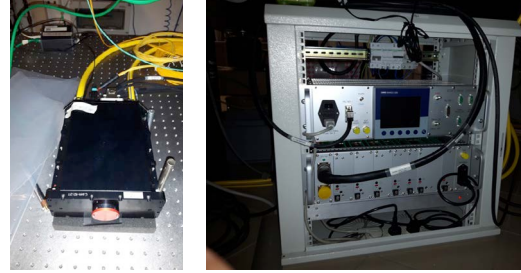
Figure 10. One of the two WFS cameras and the related electronics in Arcetri (provided by ESO)
