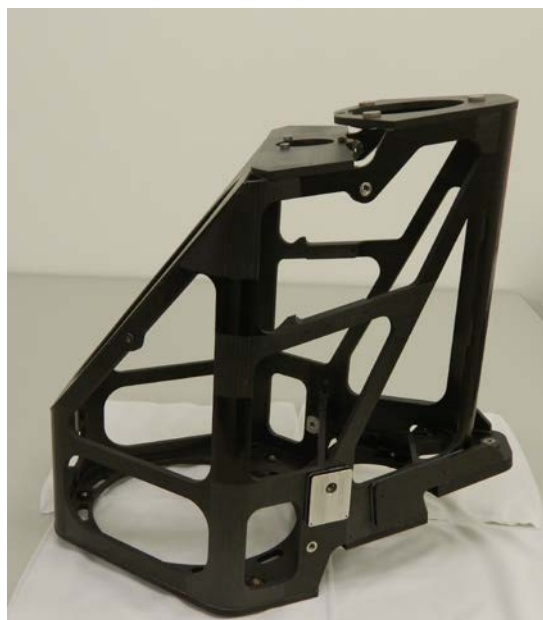
Fig. 3. CaSSIS CRFP structure
