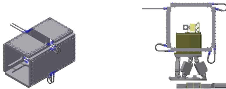
Figure 11: Thermal box. Left: schematic drawing. Right: the thermal box surrounding the MM, positioned on its interface piece, and on the motorizations.
