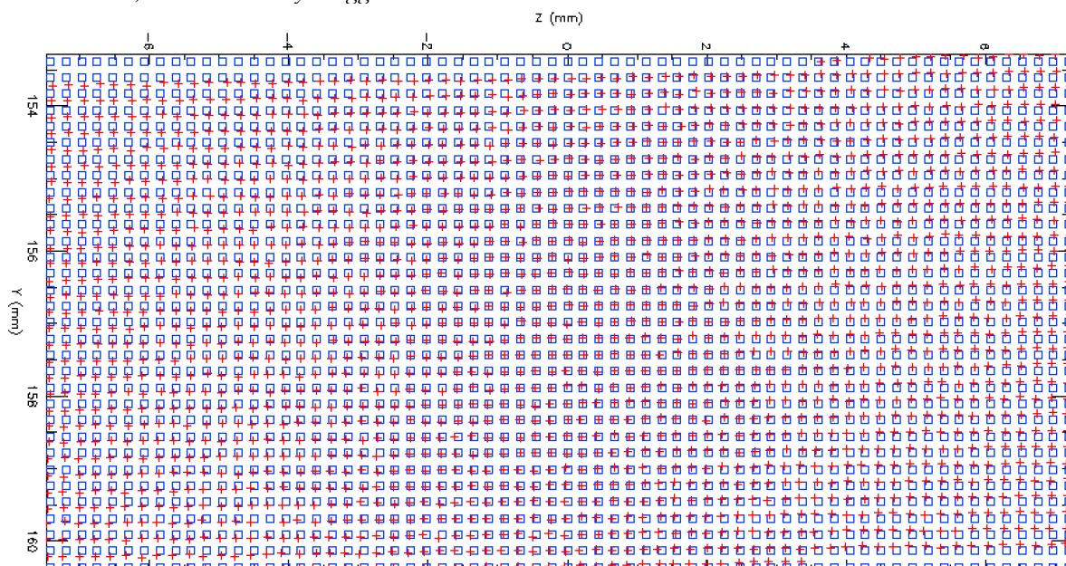
Figure 15: another simulated output of a Hartmann sensor placed after the parabolic mirror (rotated by 90 deg). In this case, we have simulated a large rotation of the paraboloidal mirror about the y-axis. The wavefront twist can be seen from the displacements of the crosshairs along the y-axis. This is exactly the effect that causes the beam intensity gradient in Fig. 7, right.
