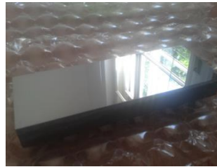
Figure 8: The beam expander in silicon for the 4.51 keV beam line. The surface has been polished to remove the lattice damage introduced by the cut (process done at CNR-IMEM). The crystal dimensions are 170 mm \times 60 mm \times 20 mm
