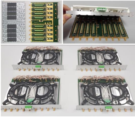
Fig. 7. Photos of the WS RF/IF module. Top left: mechanical housing (left) and fabricated PCB (right) before assembly. Microwave absorbers are glued in the pockets of the PCB mechanical housing. Top right: PCB board (first prototype version) and mechanical housing during assembly with optical transmitters. Bottom: Four WS RF/IF modules fully assembled, with OTXs.
