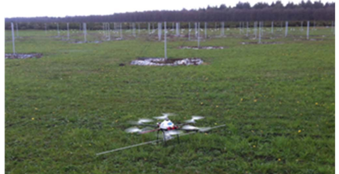
Fig. 1. Partial view of the LBA array. The UAV equipped with a 2-m long dipole is taking off
