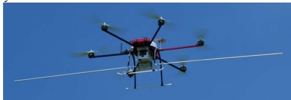
Figure 1: UAV-based flying test source. The payload consists of a GNSS receiver, an RF generator and a dipole antenna.
