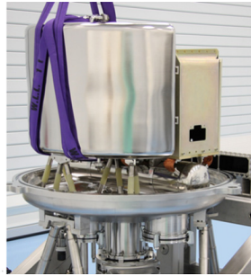
Fig. 19: IRDIS opto-mechanical layout (left), and picture of the IRDIS cryostat during integrations (right).
