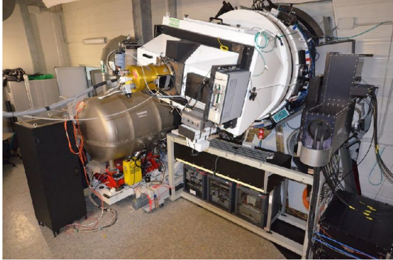
Figure 1. Picture of the current configuration of the Nasmyth-B focus of TNG. Left : the electronics and the dewar containing GIANO-B, mounted on a dedicated platform. Top center : the Low Resolution Spectrograph (LRS) that hosts the entrance slider where is located the dichroic. Bottom center : the new GIANO-B preslit that receives the light through LRS. It is mounted inside the lodgment of SARG (the previous high-resolution spectrograph of TNG) together with the corresponding electronics. Right : The front-end and calibration units of HARPS-N.
