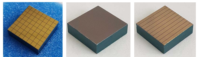
Figure 4. (left) Original CZT crystal tile; (center) final anode side configuration; (right) final cathode side segmentation.
