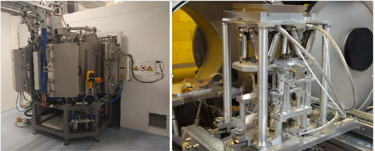
Figure 5: Tools are very important, preparing the way to the implementation phase. The coating and stacking of the mirror plates requires a high level of automation, in order to satisfy the programmatic requirements of the ATHENA mission. An industrial coating machine is being commissioned at the premises of the main SPO contractor, cosine (left). The assembly of the mirror plate stacks into mirror modules is a precision operation, taking place at a synchrotron facility. A dedicated 24 DOF assembly tool was developed and installed at the XPBF 2.0 beamline at the BESSY II facility in Berlin, Germany, consisting of 3 vacuum compatible hexapods, mounted on the beamline optics chamber hexapod (right).
