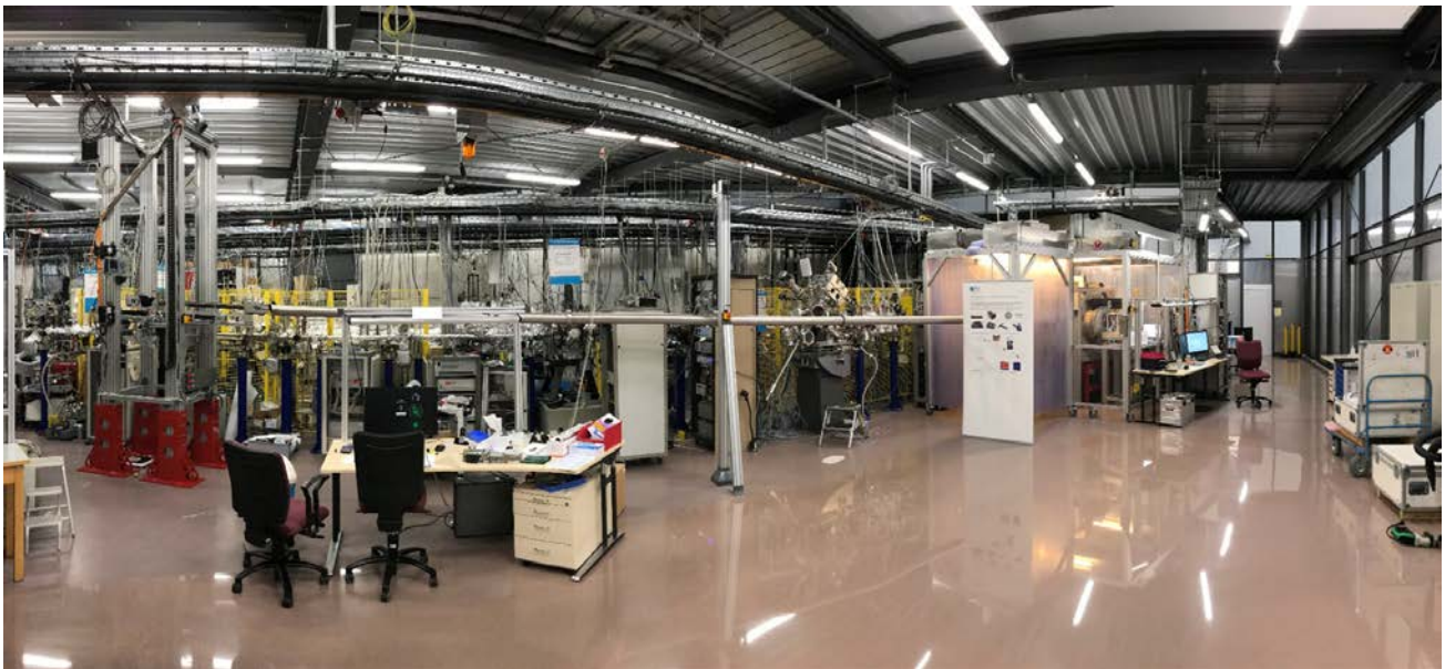
Figure 12: The MMs are assembled and characterised using synchrotron radiation metrology. The ATHENA beamline was completed and commissioned in the laboratory of the Physikalisch Technische Bundesanstalt (PTB) at the BESSY II facility in Berlin. The clean tent protecting the optics vacuum chamber is visible in the right part of the image, connected with a vacuum beamline to the focal plane assembly tower, on the left side of the image. This facility was used for the referencing of the MM for the indirect MM integration approach.
