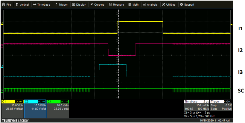
Figure 15 - Vertical waveforms without capacitor filter in the intermediate board
