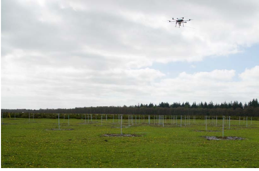
Fig. 1. UAV-based system flying during a measurements campaign on a LOFAR LBA station located in The Netherlands.
