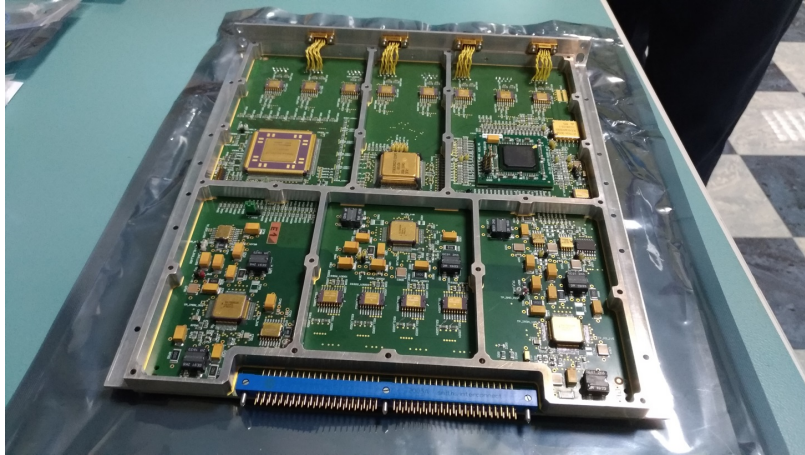
Figure 11. Router and compression unit (RDCU)
