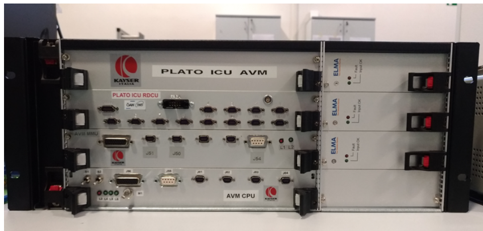
Figure 5. Avionic Model (ICU AVM)
