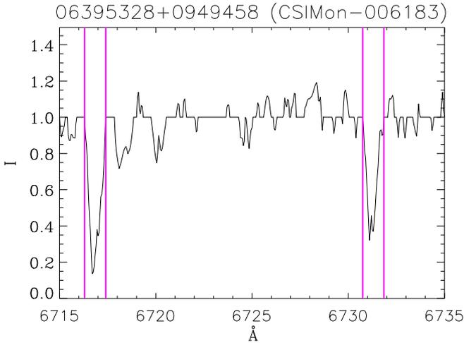
**Fig. A.2.** Range of the spectrum of one object around the [SII] doublet: our tool allows us to select those objects with spurious absorption features, as highlighted by the vertical magenta lines around the absorption lines in this figure.
