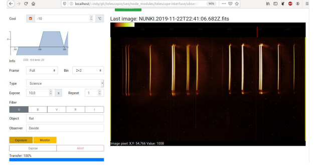
Fig. 3. Preliminary design of the web interface for the control of SBIG cameras. In this image, the SBIG STL 11000M camera is used to take a Neon-Argon lamp calibration frame for the LHIRES III.
