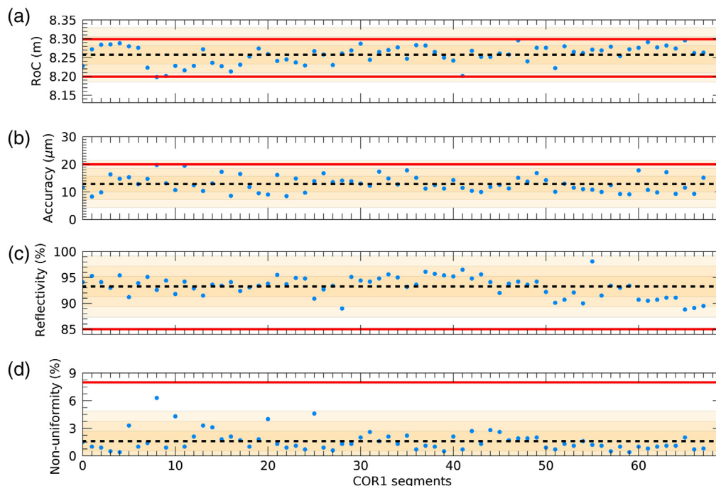
Fig. 10 Main parameters of the COR1 segments of ASTRI M1 from the first (segment 0) to the last made (segment 67): (a) radius of the spherical component, (b) residual shape error, (c) average reflectivity, and (d) reflectivity nonuniformity. For each panel, the solid red and dashed black lines represent, respectively, the applicable requirement value and the average value.
