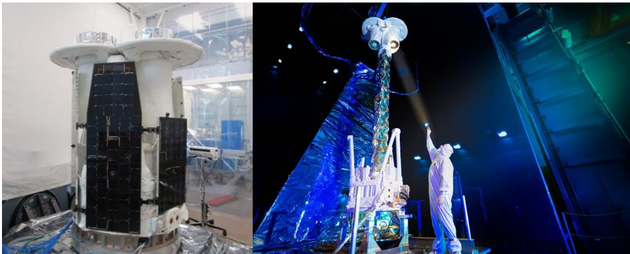
Figure 10: IXPE observatory on vibration table (left) and being prepared thermal vacuum testing (right). Credit: Ball Aerospace.
