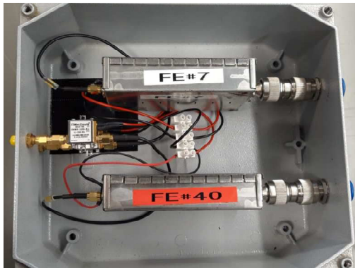
Figure 2. Photo of the box containing two BEST front-end (FE#7 and FE#40), one for each Vivaldi antenna channel. Each BEST front-end is directly connected to a Bias-Tee that provides the 12 V power supply [16-17].
