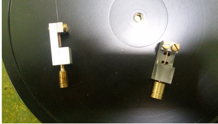
Figure 3: Squeezing blocks used to terminate the W fibers
