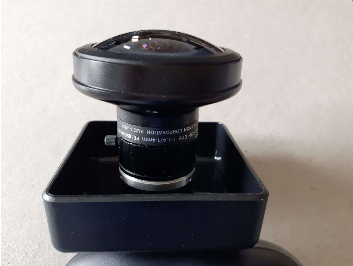
FIGURE 4.1 THE FUJINON FE185C046HA-1 FISH-EYE LENS USED IN OUR TEST
