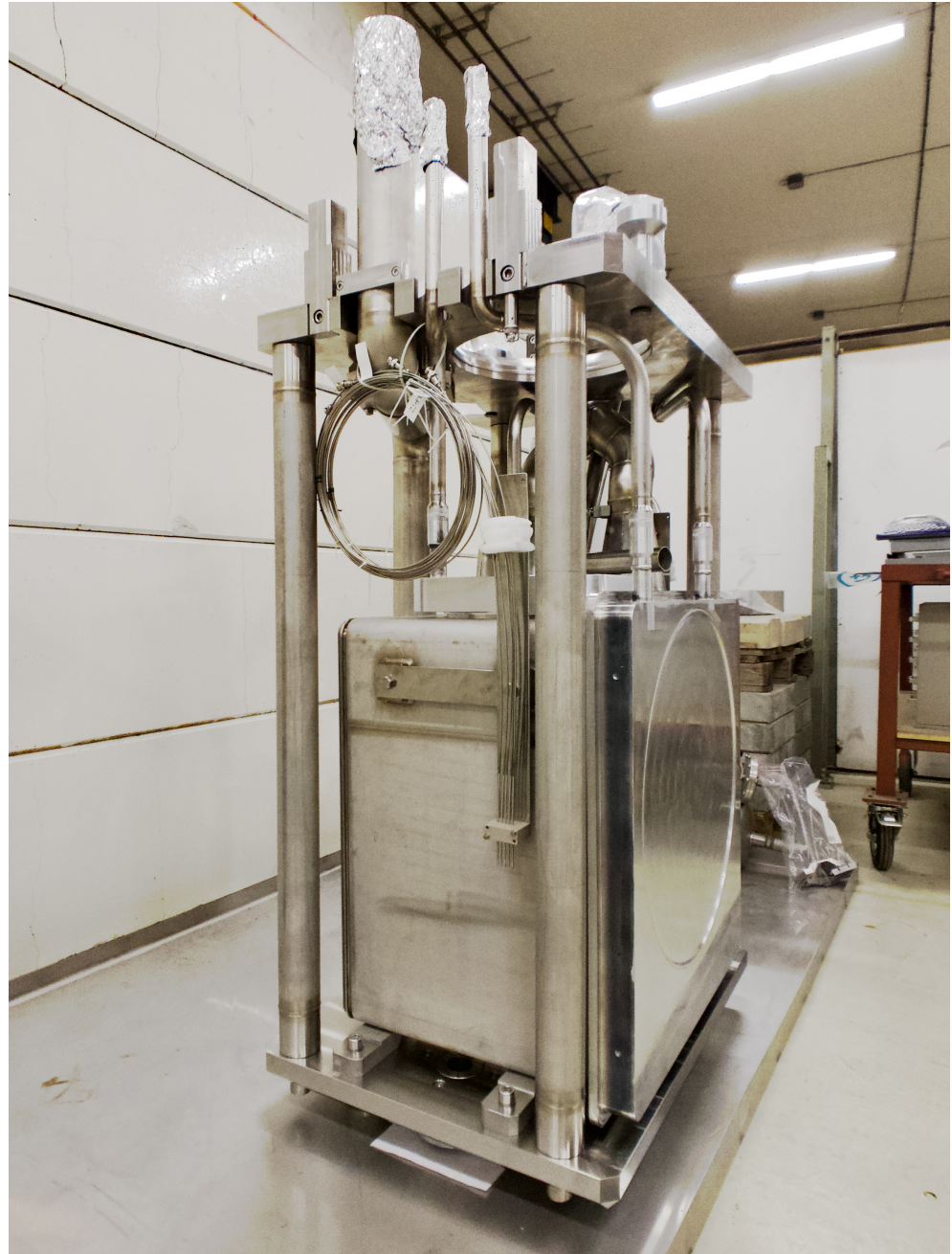
Figure 3. The n_{TOF} spallation target during the installation phase. The right side station with 5 SPNDs is visible at the centre of the photo.
