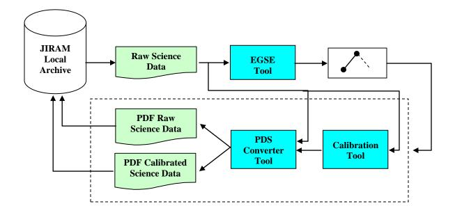
Support Tools: EGSE (delivered by GA). PDS Converter. Calibration Tool
