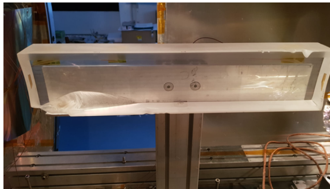
Figure 1: the paraboloidal mirror of BEaTriX in the IBF facility of INAF-OAB, prior to a figuring run of the surface. The broken or chipped parts are outside the optically-finished areas and will not be used in operation, or in tests at PANTER.
