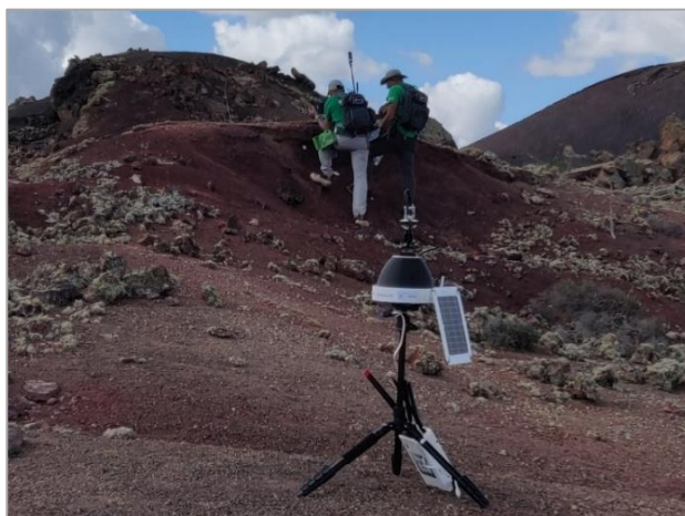
Fig.2: OMNICAM deployed in the field in an ESA Analogue Astronaut Training Campaign.
