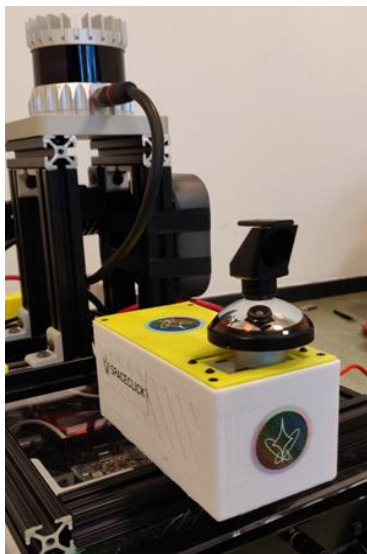
Fig.4: OMNICAM integrated in a rover part of a monitoring, mapping and sampling swarm, and tested at the ESA-ESRIC robotic challenge 2021.
