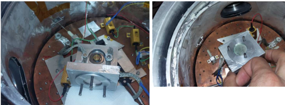
Figure 23: Images of the dewar and the surface of the ZnS T dichroic after the disassembly procedure.
