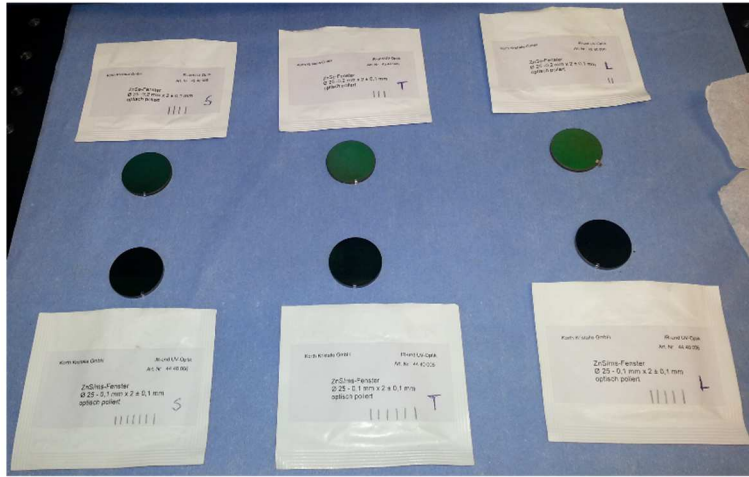
Figure 1: a picture of the ZnSe (on top) and ZnS (on bottom) dichroics filters.
