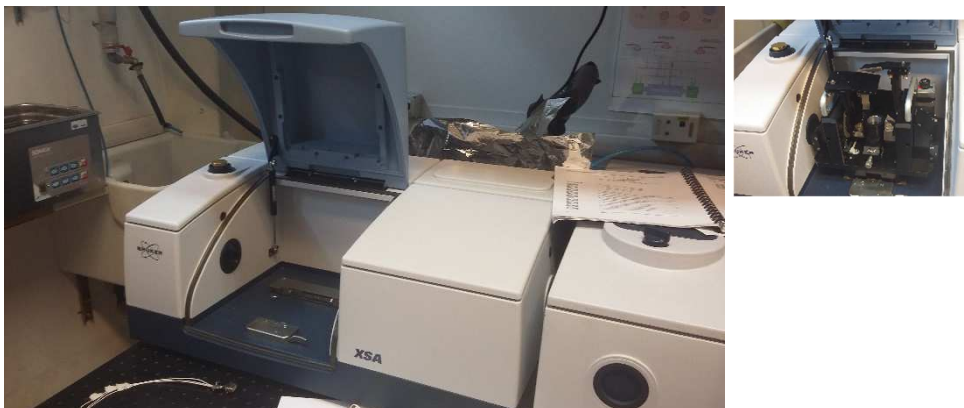
Figure 4: FT-IR spectrometer (on the left) and the optical setup used to recorded the reflectance
