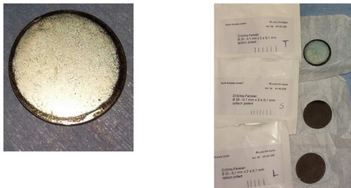
Figure 24: Images of the ZnS T dichroic after the second irradiation test (on left) and a comparison with the other dichroics on the right.
