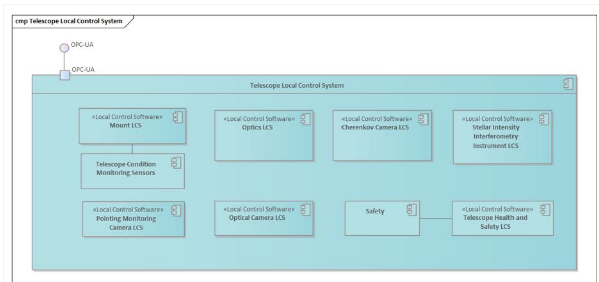
Figure 14: Telescope Local Control System's main Local Control Software.
