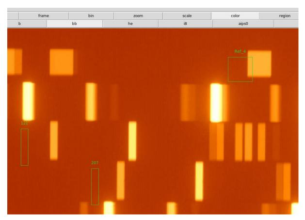
The first time, usually slits will not be in the proper position, we have to tune the model moving<sup>1</sup> these slits on the expected reference line position<sup>2</sup>, using the standard DS9 regions commands
