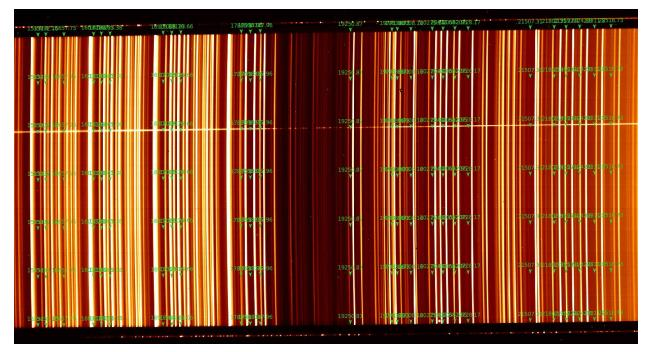
The same line position is showed 7 times along the slit. Adjusting the line position for each piece, we will instruct the model to follow the lines curvatures<sup>9</sup>
