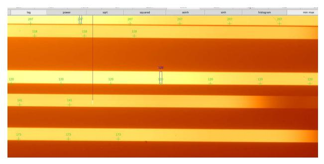
DS9 will show the slits position (the blue region) and 9 crosses for each slits along the expected position of the spectra traces. Like we did for the OPTMode1, we must adjust in DS9 the crosses along the *left side* the spectra traces.<sup>5</sup>
