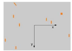
The OPTModel locates the mask slits on the FOV. Since we are working with dispersed images, slits are not visible on the frame. For this reason we will use an arc frame to tune the model: we will use the lambda reference position on the frame as *virtual slit*.
