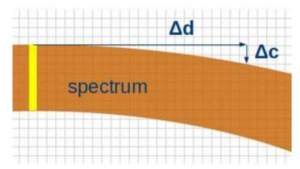
Each slit has own set of  $c_{x,y,i}$  coefficients, different slit by slit, because each slit is in a difference position in the FOV. SpectraPy uses a global model to describe coefficients variation along the FOV.
