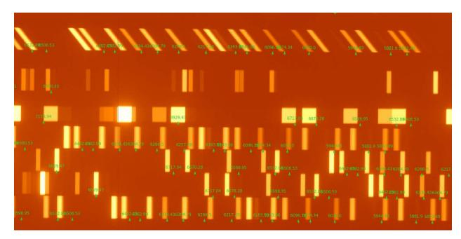
The method plot\_ids\_model displays the frame and over it, green arrows on the expected line positions. For each list, we must move the arrowhead in the proper position and then refit the model. In this figure we can see how arrow positions don't match the line positions. The adjustment is not a simple global shift, we are suppose to adjust the model slit by slit, since the distortions are different along the FOV. Moreover each arrow position on the slit, must be moved of a different amount.
