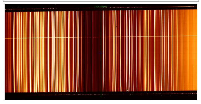
In this case we have just one slit, and the slit mutal positions can not be used to derive the scaling factor of the Optical Model. You can see how the nominal scale factor is not enough accurate since the slit size (green box on the frame) doesn't fit the size on the dispersed frame.
