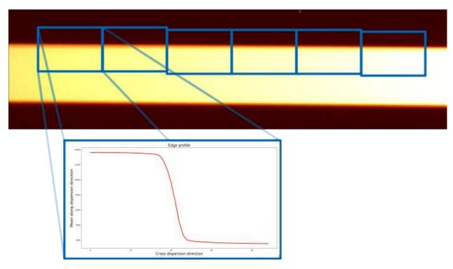
The TraceCalibration class is the object used by SpectraPy, to fit the edge of the spectra trace
