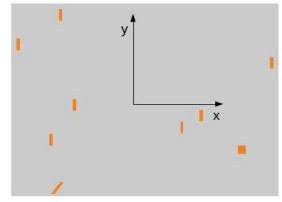
As we can see, in this case the mask and the image don't match, slits are not in the expected position, we can check this discrepancy looking at the tilted slit or at the reference square slit.
