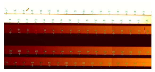
For visual check, SpectraPy displays in DS9 the computed edges. It places green crosses on the computed edge positions. It also shows red crosses in case of failures.
