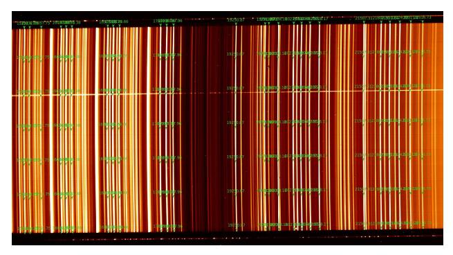
Once done, we refit the model and check the solution on the frame. We can also increase the number of slits for a better check.
