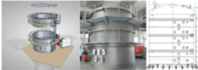
Figure 1-8: Image for refer. only: example door on the top of the vessel for positioning of the DUT.
