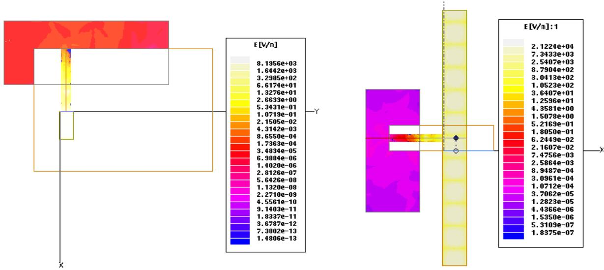
Figure 10 E-total Field representation on a cut-plane [x-y] passing through the hole's axis. The colour scale is logarithmic
