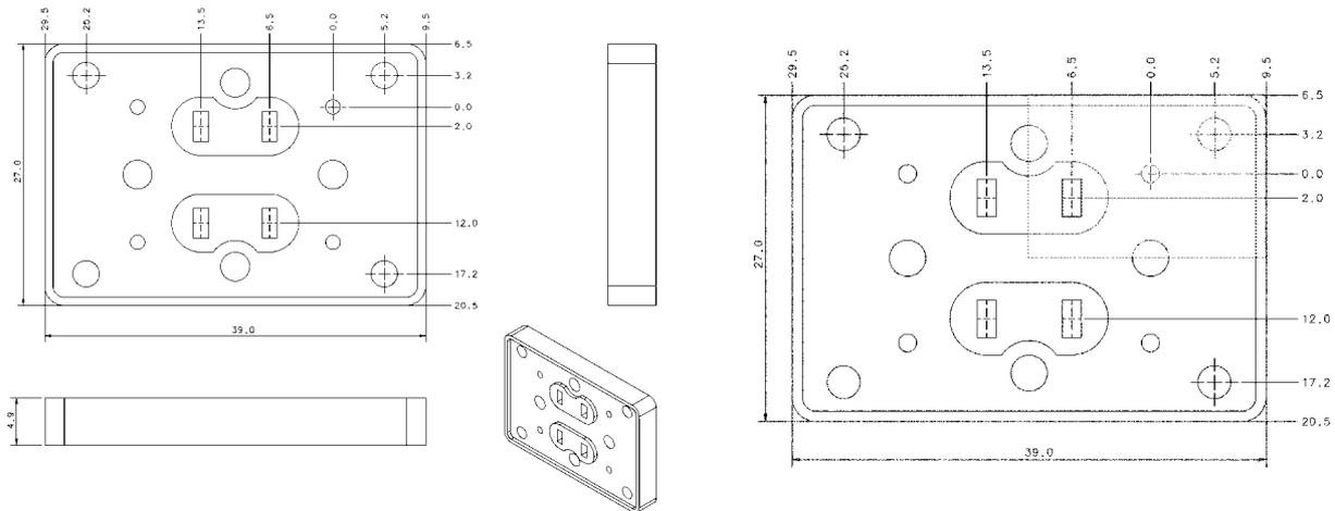
Figure 2: 70 GHz flange design adopted for these simulations (left). The electromagnetic model has been defined assuming the shadow part as reported in the right panel:  $\frac{1}{4}$  of the geometry has been used.
