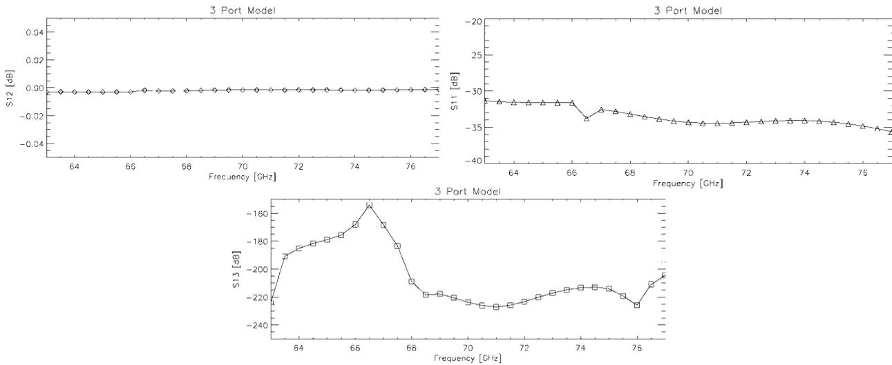
Figure 5: Scattering Parameters in dB as a function of frequency. Upper left:  $S_{12}$  (waveguide insertion loss). Upper right:  $S_{11}$  (return loss at the waveguide input port). Bottom:  $S_{13}$  (Insertion loss between the waveguide input port and the hole).
