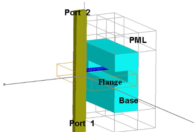
Figure 7 3-D rendered representation for the two ports model 2; in evidence as flat shaded, the waveguide (green), the hole (blue), the base (light blue); represented as wireframe are the flange (brown) and the PML boxes (grey)
