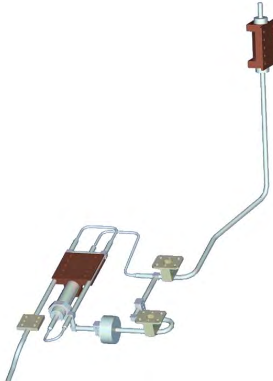
Figure 2-5 Sorption Cooler Cold End
