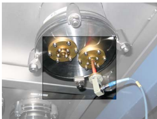
FIGURE 3: LEFT – DETAIL OF THE COAX – WG TRANSITION CONNECTED TO THE FEED THROUGH BY A WAVEGUIDE SECTION; RIGHT – DETAIL OF THE FLEXIBLE WAVEGUIDE END
