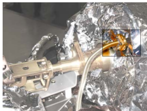
FIGURE 3: LEFT – DETAIL OF THE COAX – WG TRANSITION CONNECTED TO THE FEED THROUGH BY A WAVEGUIDE SECTION; RIGHT – DETAIL OF THE FLEXIBLE WAVEGUIDE END
