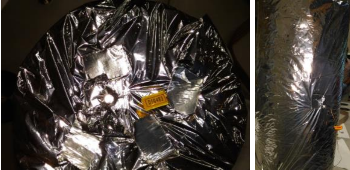
Figure 4 Locations of the G (left panel) and H (right) sensors on the top and the side of the shield covering 4K stage, respectively.
