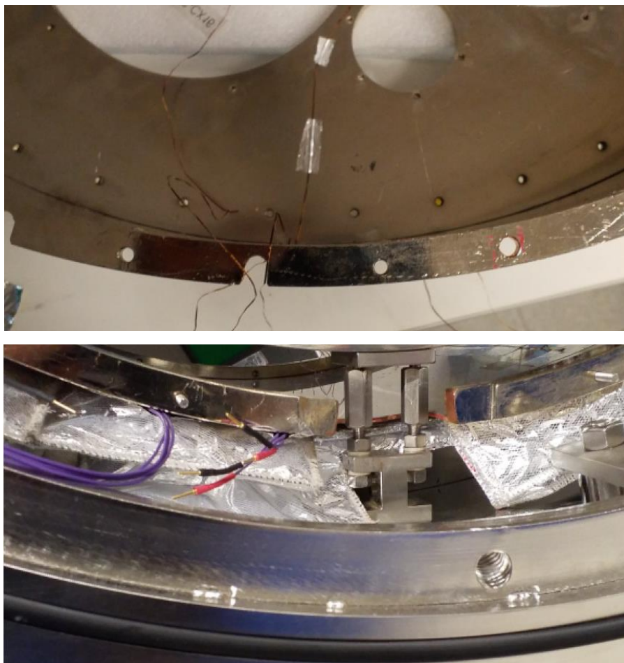
Figure 15 thermometers wires: 2 X4pin connectors are used to connect the manganine wires of the thermometers placed on the IR filter holder to the copper wires (violet, bottom picture) connected to the L-shaped connectors supports.
