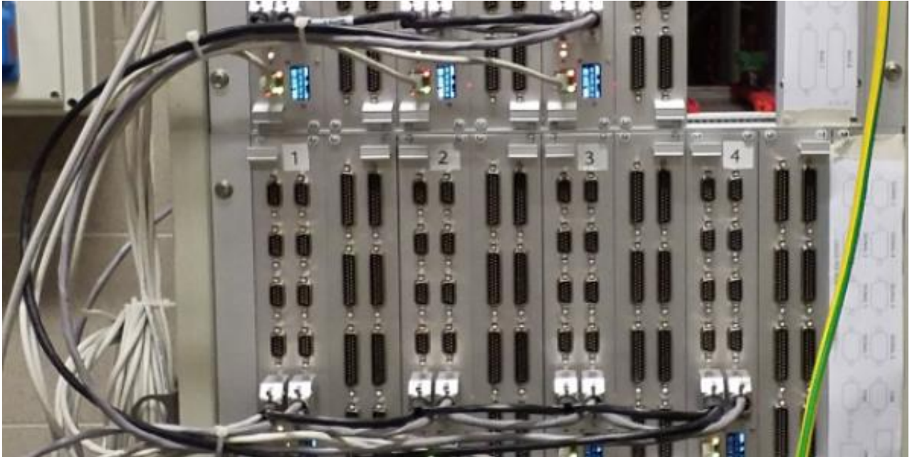
Figure 28 : CAN (black) / SYNC (grey) harness: connection scheme. All the board are connected in parallel to the SYNC/CAN external box.
