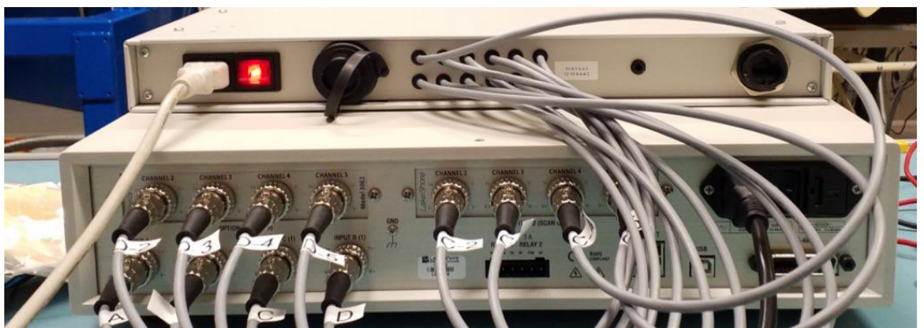
Figure 25 Harness from Multiplexer to Lakeshore. Labels are reported in §0
