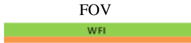
Figure 3: : a passivation layer (orange) can be deposited on the non-illuminated side of the detector.
