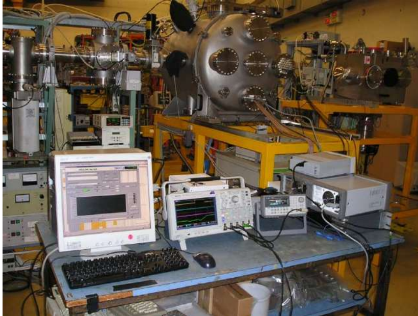
Figure 4-20 The measurement setup in front of the vacuum tank (on the background, already closed). On the table, from left, there are the PC with the LabView software, the digital oscilloscope for waveforms control, the PXI chassis (barely visible behind the oscilloscope), the signal generator and the power supplies.
