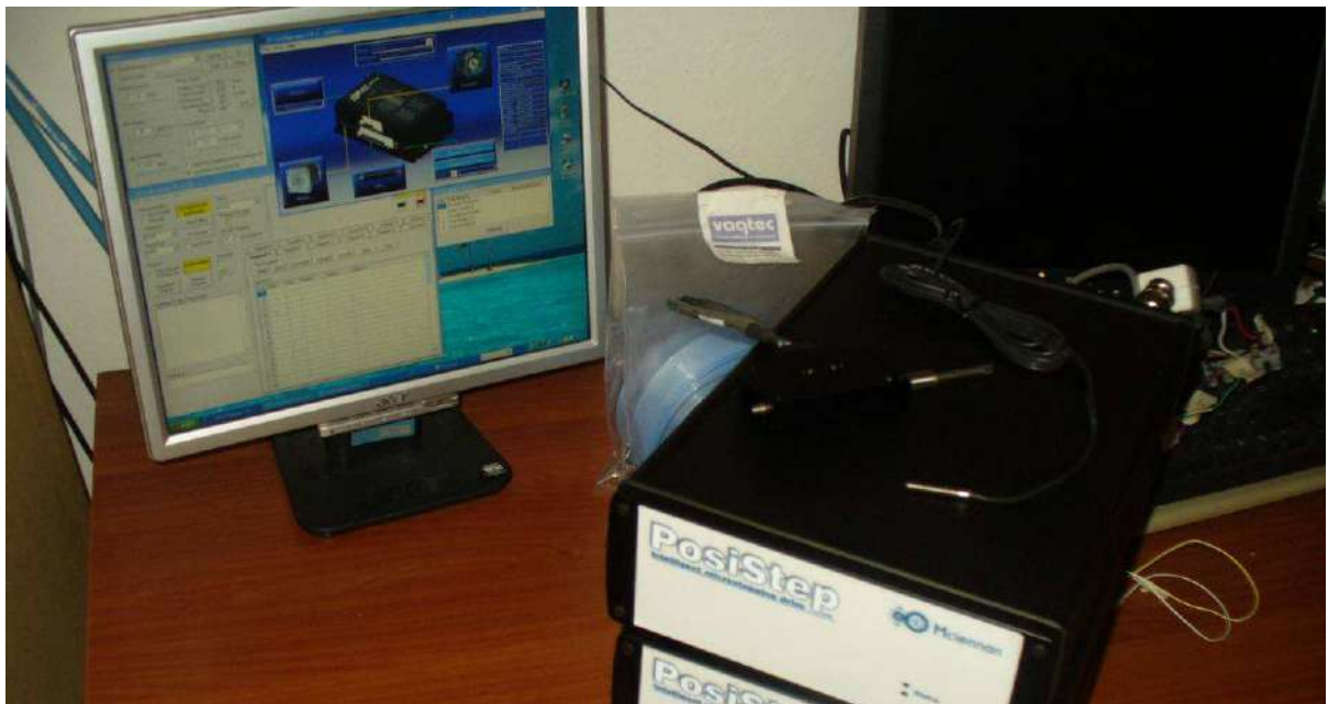
Figure 6-16: Some electronic components of the jig under test: linear encoder and proximity sensor are visible on the electronic box. The control is made by computer.
