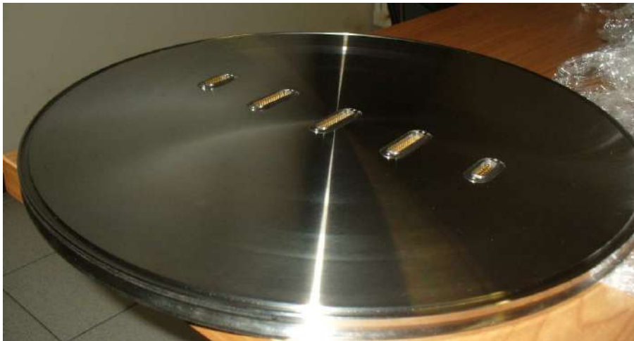
Figure 6-18: PANTER flange with dedicated connectors
