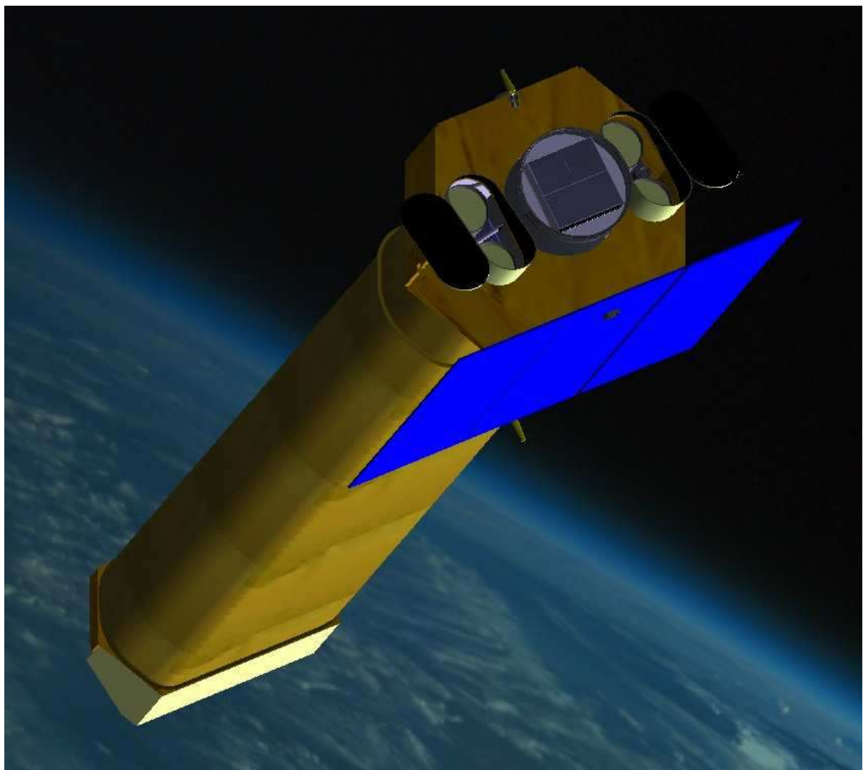
Figure 2-1: artistic view of the NHXM satellite. The four mirror modules are on the satellite platform (top right corner in this figure) and the focal plane cameras on the detector platform at the end of the deployable truss (lower left corner).
