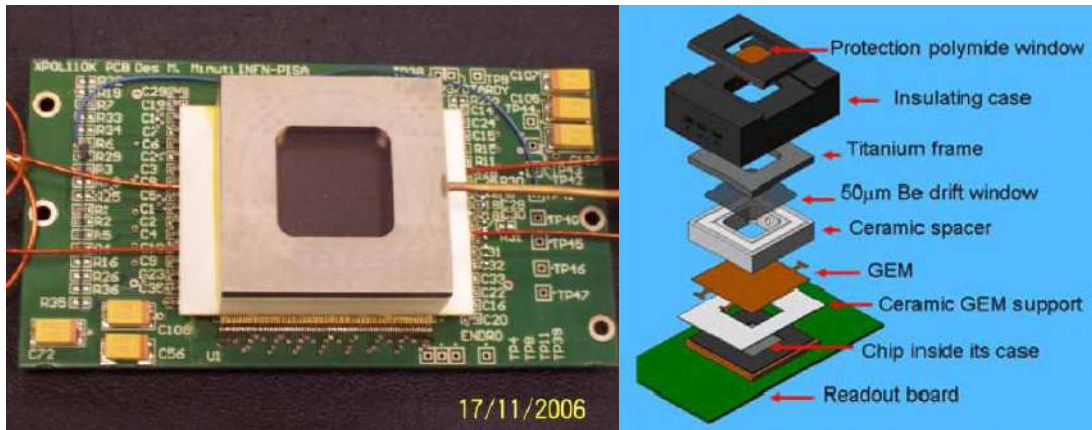
Figure 5-5: The LEP Detector-FEE Assembly
