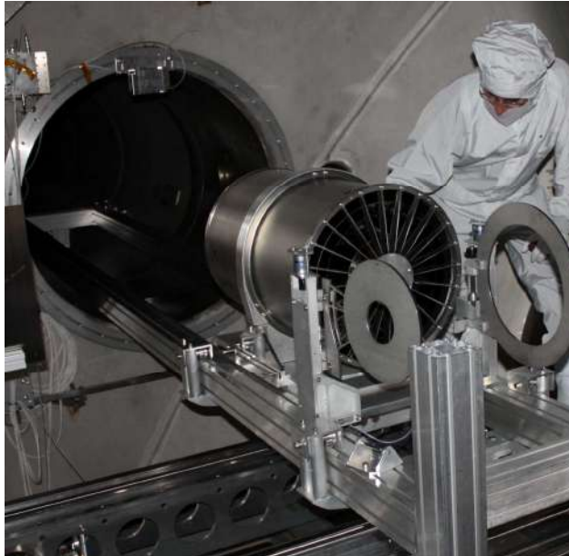
Figure 3-14: a mirror module prototype, including a W/Si multilayer-coated mirror shell, tested at PANTER. The focal spot seen in the TRoPIC CCD detector in a X-ray energy band of 20-35 keV. The HEW is 22 arcsec, very close to the specification (< 20 arcsec for E < 30 keV).
