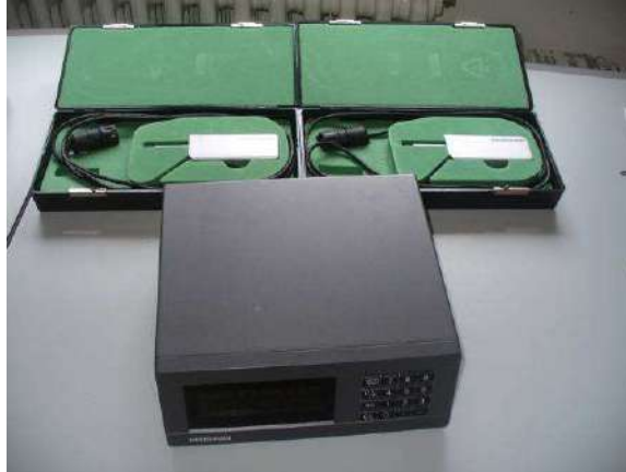
Figure 6-17: Heidenhain sensor for the rotation calibration
